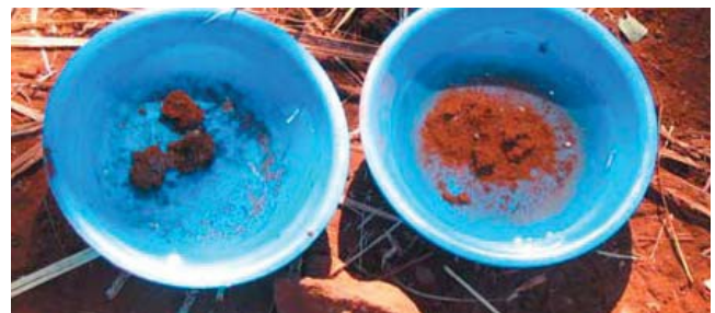
Figure 3: A field-test of aggregate stability. Small clods from a ploughed field (right) and virgin land (left) have been dropped carefully into water. The lighter coloured clods from the ploughed field disintegrate, while the clods from the virgin soil stay intact.
